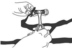
Insert the cushion onto the mask frame. Ensure that the bulge on the main frame embeds into the notch on the cushion.
