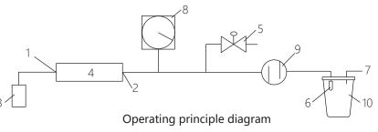
1.Exhaust outlet 2.Suction inlet 3.Silencer 4.Vacuum pummp 5. Negative pressure regulating vavle 6. Overflow valve 7. To phlegm suction catheter 8. Vacuum meter 9. Air filter 10. Liquid holder
